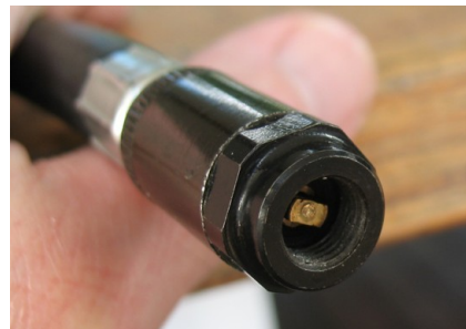
Fig. 2 Show brass part that opens Schrader valve
