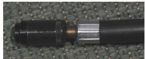
Fig.3 Fitting wound out allows Schrader valve to close.
