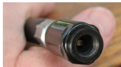
Fig. 4 Centre brass fitting in retracted position.
