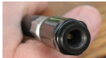
Fig. 4 Centre brass fitting in retracted position.
